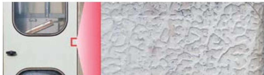
*Ultra-long life anywhere! This Intertec cabinet's gel-coat survived 40 years in an atmosphere containing sulphuric acid; the surface (right) is still intact with only minor thinning.*
