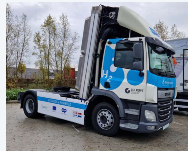
VDL Prototype Truck 44t 4x 50kW Fuel Cell, 40kg/350bar H2 Tank System, 210kWh Battery
