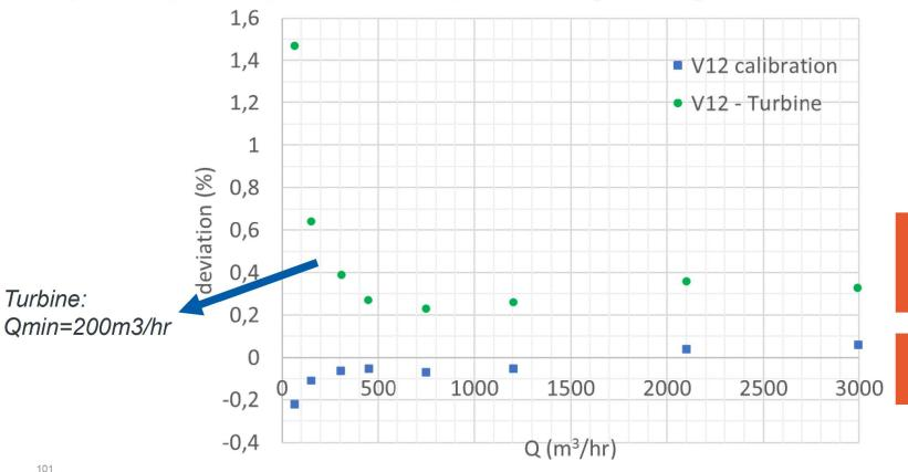
Baseline curve determined for deviation of Turbine vs. V12 on natural gas
