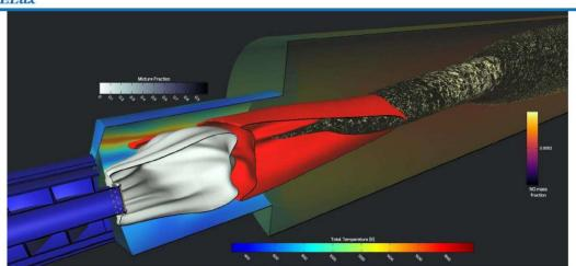
White = the fuel volume injection just before igniting. Red = the stoichiometric point of the mixing, and it is contoured with the temperature Black & Yellow = the thermal NOx source which starts from inside of the root flame and continues to the end of the chamber. For that, the yellow-purples scaling is foreseen in the right side of the figure. How starts the combustion, ignite and also flame definition and the tracking of the NOx source.
